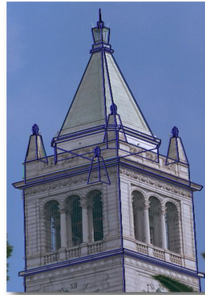
Model edges projected onto photograph
